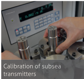
Qualification of the subsea components
