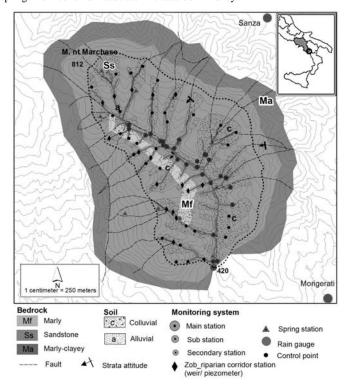
Figure 1. Location and geomorphological map of the Ciciriello Experimental Catchment (from Cuomo and Guida, 2016 under revision). Legend: Bedrock lithology; Ma: Marly-clayey and argillitic tertiary formation, base aquiclude; Ss: Sandstone Miocene formation, fractured general aquifer; Mf: Marly limestone, interlayered and perched aquifer.
