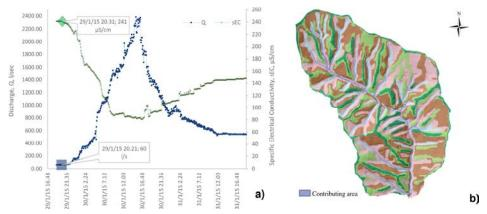
Figure 9. a) Pre-event hydro-chemograph conditions, just before the storm event, with Q=60 L/s, filled blue square and EC=240  $\mu$ S/cm , filled green diamond, b) scenario corresponding to groundwater and decreasing groundwater ridging contribution to streamflow running exclusively along the riparian corridor and main streamflow.
