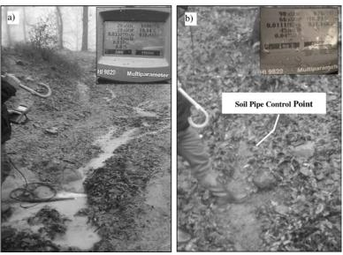
0 Figure 5. Measurements at 12:00 am in the dirty road point controls (a) and the soil pipe (b) with respective sEC measurements.
