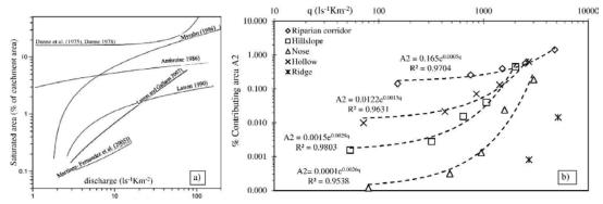
Figure 15. a) Relationship between the total extent of contributing saturated areas and the baseflow discharge in several small (less than 10 km²) catchments (modified from Latron and Gallarat, 2007); b) Relationship between the contributing areas and the specific discharge for each hydro-geomorphotypes of the Ciciriello catchment.
