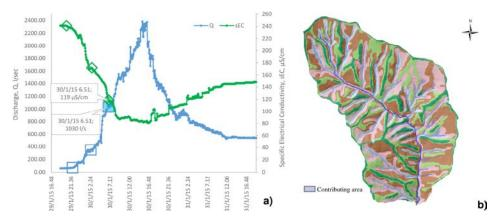
Figure 11. a) Progressive hydro-chemograph conditions, after approximately 60 mm of rainfall, with approximately Q = 1000 L/s, filled blue square and approximately  $EC = 120 \,\mu\text{S/cm}$ , filled green diamond, b) scenario corresponding to a full saturation excess contributions to streamflow along the riparian corridor and at transient channels within the colluvial hollows, respectively.
