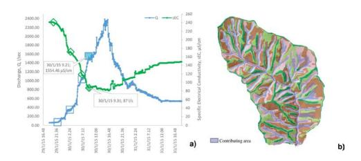
Figure 12. Advanced hydro-chemograph conditions, after approximately 80 mm of rainfall, with approximately Q= 1550 L/s, filled blue square and approximately EC=90 µS/cm, filled green diamond, b) scenario corresponding to a full saturation excess contributions to streamflow along the riparian corridor and the whole colluvial hollows, respectively.
