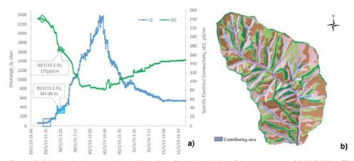
Figure 10. Initial hydro-chemograph conditions, just after the beginning of the storm event, with Q=350 L/s, filled blue square and  $EC=170 \,\mu\text{S/cm}$ , filled green diamond, b) scenario corresponding to an increasing groundwater ridging and initial saturation excess contributions to streamflow. The first occurs along the riparian corridor, the second at the apical transient channels just downstream the colluvial hollows, respectively.
