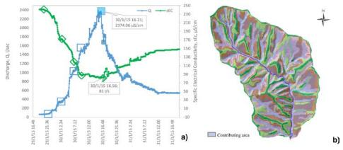
10 Figure 13. Final hydro-chemograph conditions, after approximately 100 mm of rainfall inducing a peak discharge approximately Q= 2400 L/s, filled blue square and about EC=80 μS/cm, filled green diamond, b) corresponding both to full saturation excess contributions to streamflow from the riparian corridor and colluvial hollows, as well as to macropore (soil pipe and fracture) and excess infiltration, on noses and partially on the ridges respectively.
